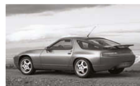
928 GTS marked by wider wings and 350hp V8
